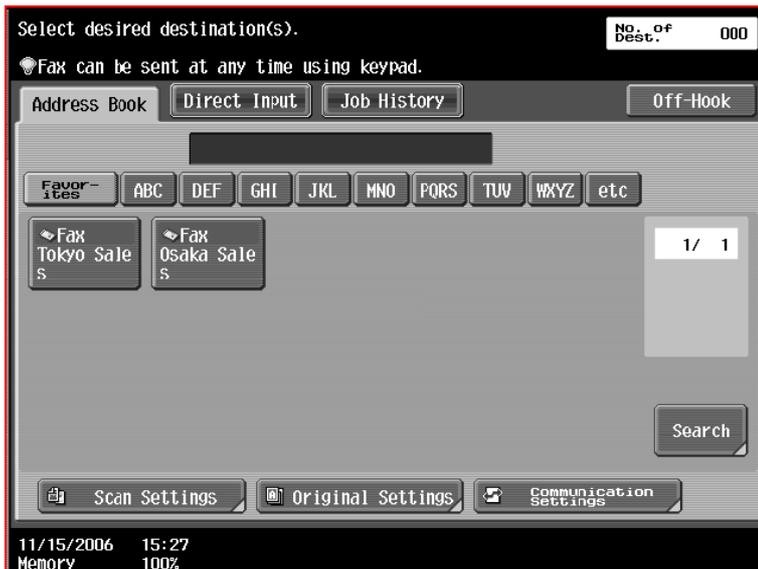
Using the keypad, enter in the fax number, or select a pre-programmed number on the screen
