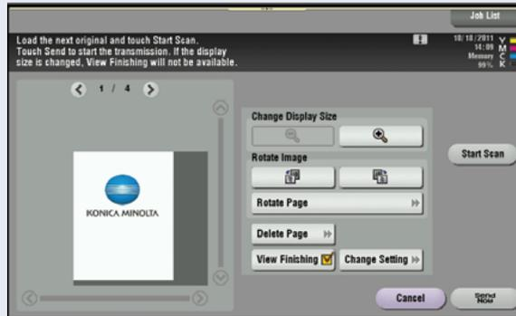
5. Touch **Start** on the **Touch Panel** or press the **Start** button. Observe that the image on the screen is the 4 originals that were just scanned. Scroll through the pages on the screen.
